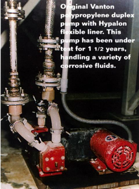
Original Vanton polypropylene duplex pump with Hypalon flexible liner. This pump has been under test for 1 1/2 years, handling a variety of corrosive fluids.
