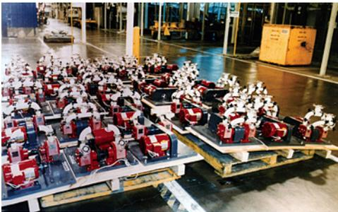
These 35 Flex-i-Liner® Duplex Teflon Pumps with Viton flexible liners are scheduled to replace the troublesome diaphragm pumps at Boeing's Wichita, Kansas facility. They will be handling a variety of acids, caustics and solvents.
